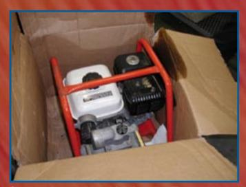
Generator that was shipped full of gasoline. The gasoline leaked out during processing.
