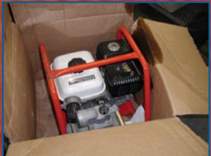
Generator that was shipped full of gasoline. The gasoline leaked out during processing.
