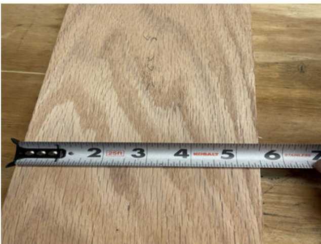
In my picture, I have a board that measures 5 \frac{1}{2} inches across
