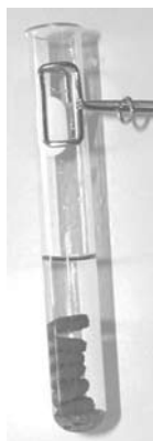
Figure 10: Copper wire and silver nitrate reaction
