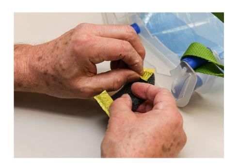
If there is adhesive on the edges of the split foam bumper pieces, remove protective film from one side.
