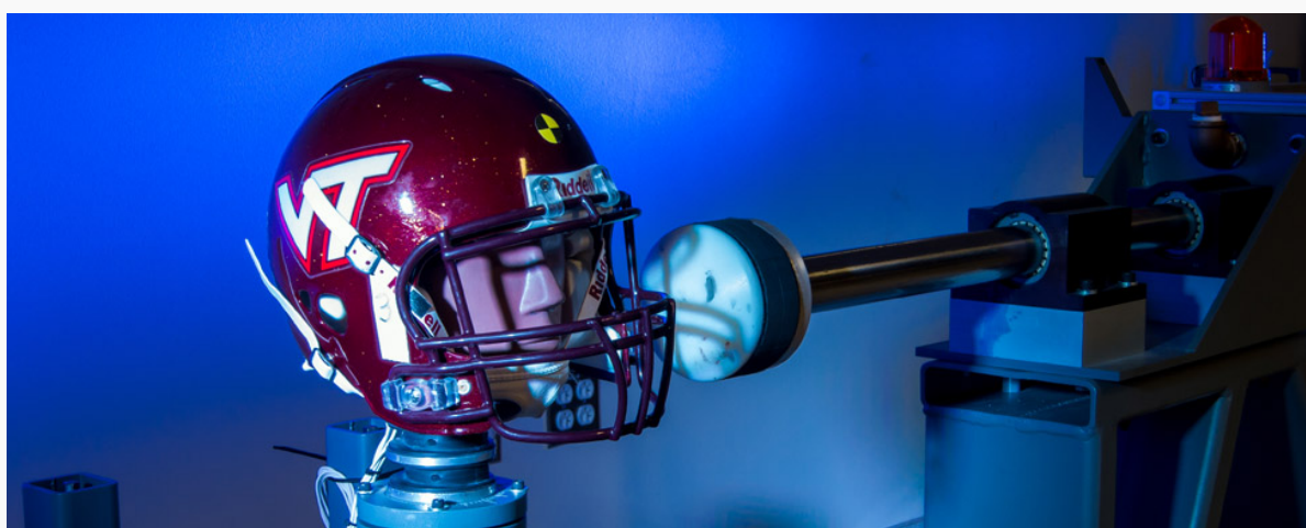
Scientists are studying the brain and helmets to better understand and prevent concussions. Researchers at Virginia Tech use this device to test how well helmets protect heads. Credit: Courtesy of Steven Rowson
